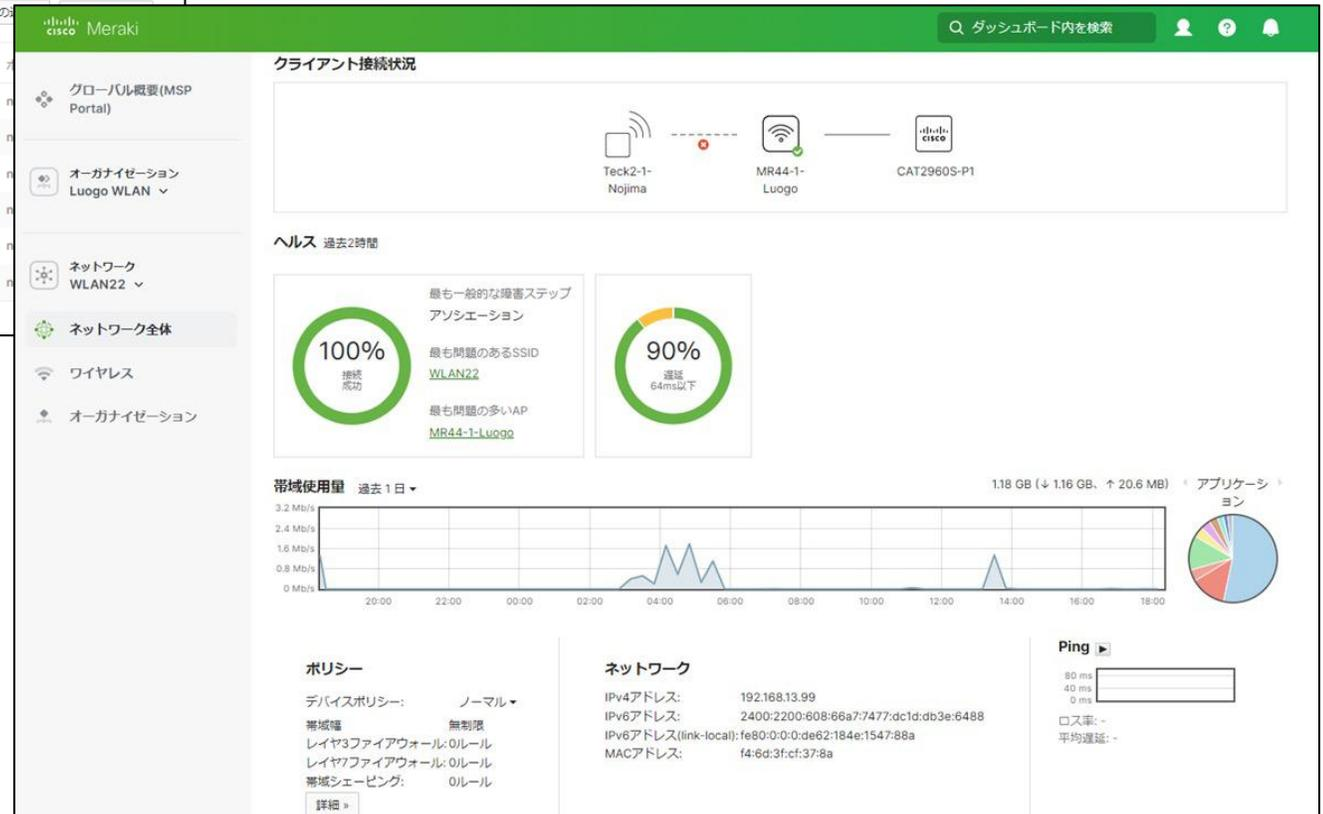
Meraki dashboard showing client connection status and health metrics. The client connection status shows Teck2-1-Nojima, MR44-1-Luogo, and CAT2960S-P1. The health status shows 100% connection success and 90% latency below 64ms. The bandwidth usage shows 1.18 GB usage over the last 24 hours.
